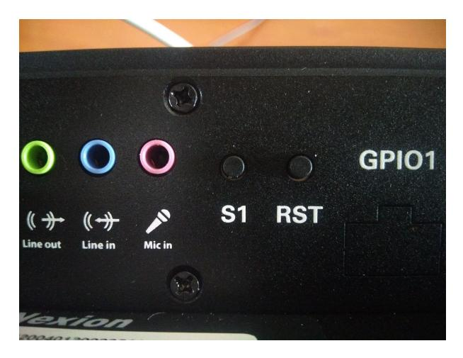
Plug the power cable into myPanel and in same time keep holding S1 button until you get into this flash menu.
